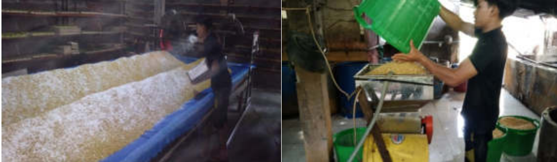
Figure 1. Process of grinding soybeans using a milling machine
