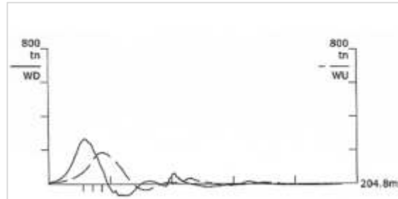
Figure 7 PDA Pile PSL 8-39 Results (Source: PT Duta Graha Karya)
