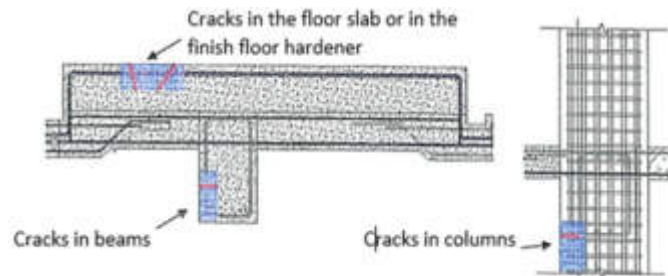
Figure 7. Parts of the structure that have suffered concrete damage Source : PT. Tatamulia Nusantara Indah
