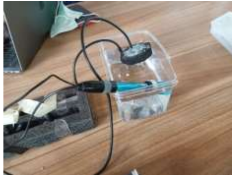
Figure 6. Sensor installation circuit for water quality monitoring applications
