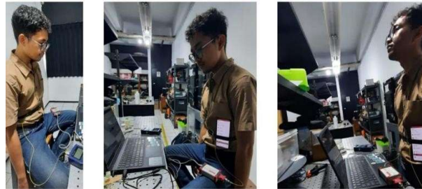
Figure 11. Set up respiratory data collection with fiber optic sensor and accelerometer sensor || (a) the research subject is seated and viewed from the right side. (b) the research subject was seated and viewed from the left side. (c) The research subject is in standing condition and viewed from the left side.
