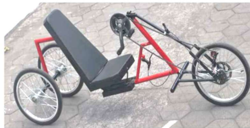
Figure 1. Handcycle for the disabled
