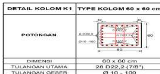
Figure 15. Details of K1 60 x 60 Column
