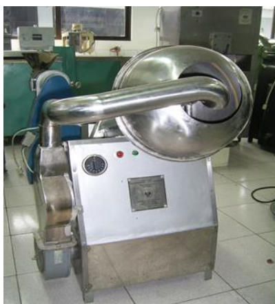
Figure 8. Mollen Dryer Construction Results
