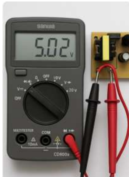
Figure 2. Power Supply Output Testing
