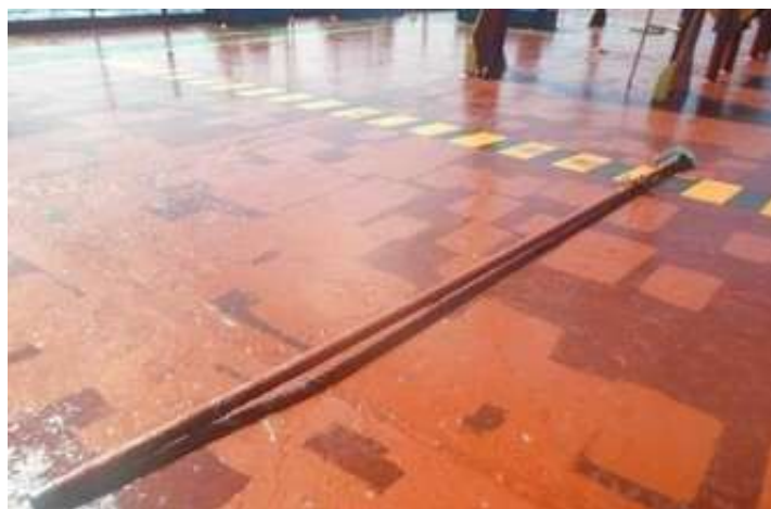
Figure 5. Removal of Hydraulic Connection Pipe Sumber : MV. Ocean Perkasa
