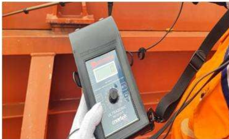
Figure 6. Inspection using an Ultrasonic Tightness Tester Source: MV. Ocean Perkasa
