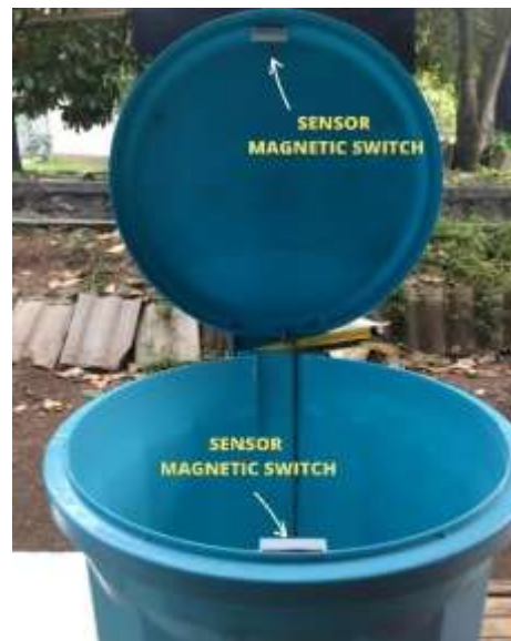
Figure 4.3 Realization of the sensor magnetic switch
