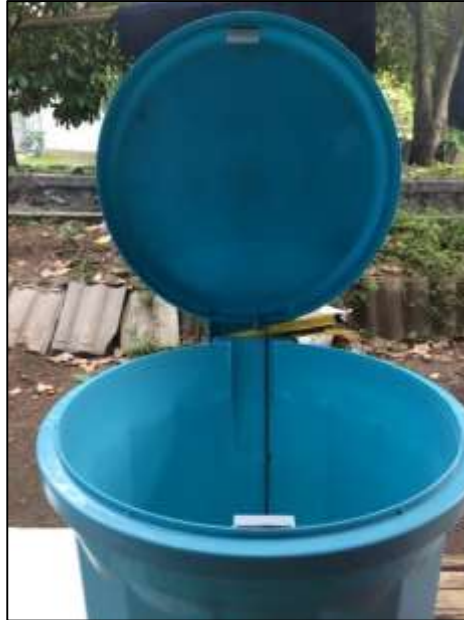
Figure 13 Sensor testing magnetic switch .
