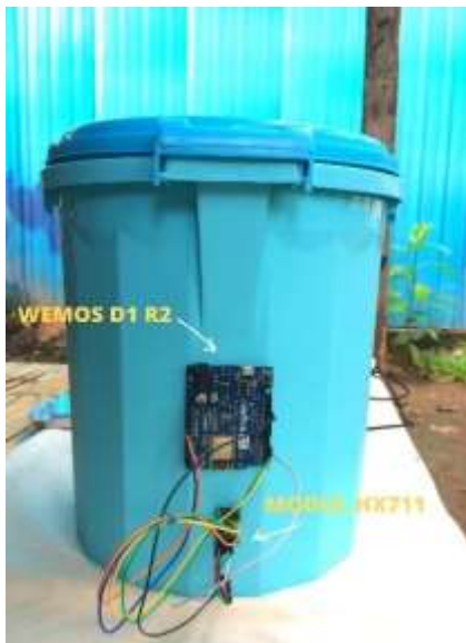
Figure 4.1 Realization WeMos D1 R2 and HX711 Module.
