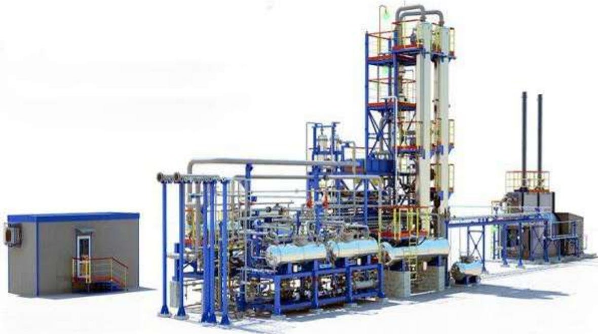
Figure 10: Mini Crude Oil Processing plant.
