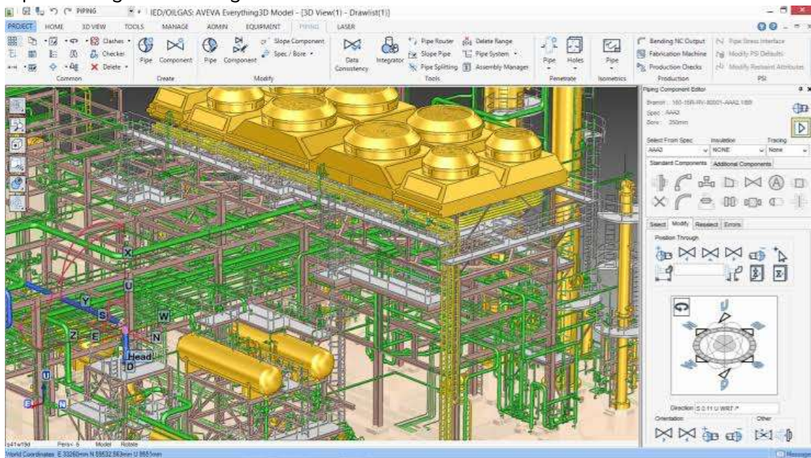
Figure 11a: The Full view of Crude Oil Processing Plant Design (Simulation) (Nnadikwe, 2023)
